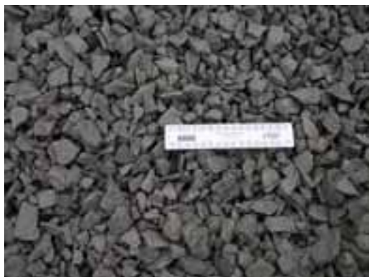
Permeable subbase (4/20 material)
